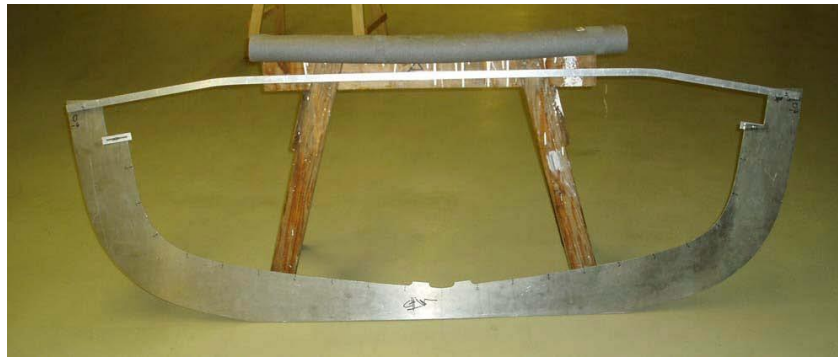
Figure H.1.5.1.2 A full section FD template made of Dural with a pinned rigid crossbar and adjustable lugs at the sheer, for alignment. However, again there is no reference line at 10 mm from the template edge. The signature shows that this template has been checked against the reference Mylar plan
