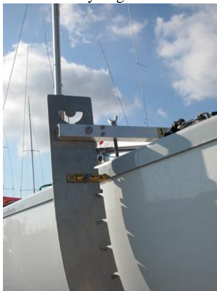
Figure H.1.5.1.1 The ISAF-produced Yngling templates showing the triangular cut outs at the measurement points and the lack of a reference line 10 mm from the template edge. The crossbeam and brass adjuster are essential added details. Note the locating pin, which precisely maintains the width of the template
