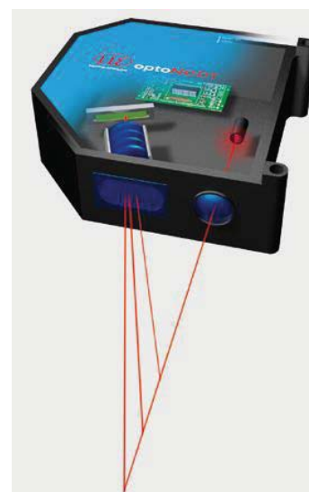
Figure F.6.2.2 A laser triangulation sensor
