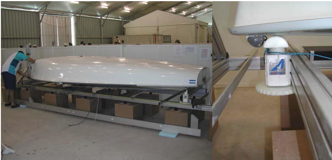
Figure H.1.4.8 Spanish 470 Jig with a hull on top (left) and the modular framing and levelling screws detail (right)
