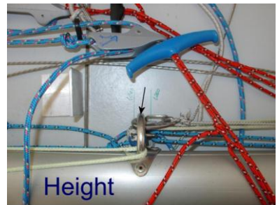
Rigging points: shroud, forestay, trapeze. Heights to be measured from MDP.
