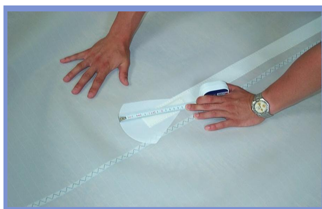
Figure K.2.4.3 Batten pocket patch size.
