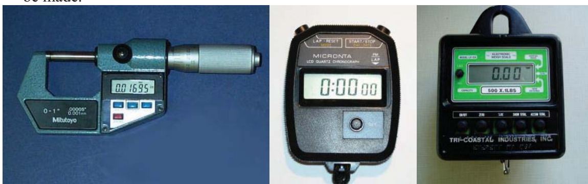
Figure F.4.8 Instrument resolution, Micrometer resolution 0.001 mm, stop watch resolution 0.01s and scale resolution 0.05 kg
