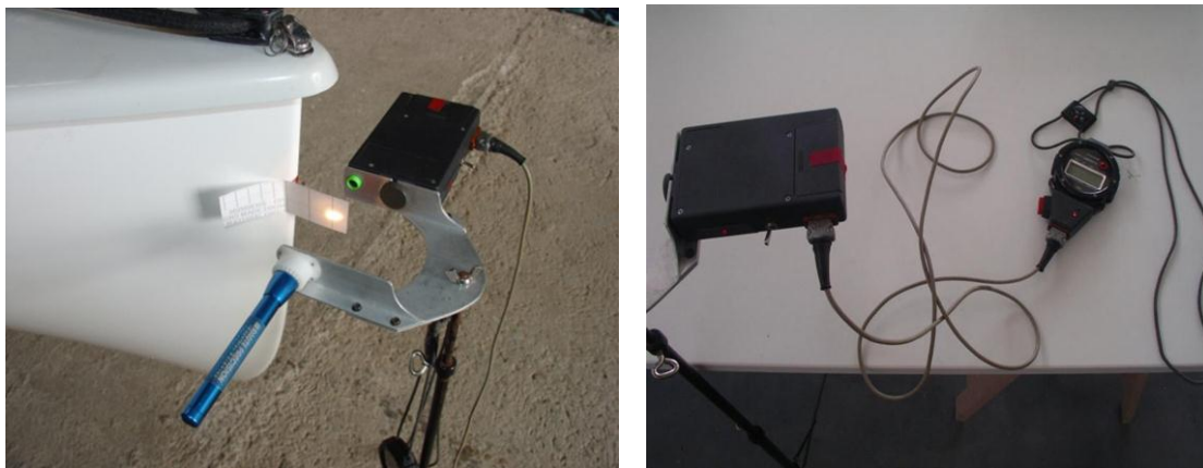
Figure H.4.2.1 A modern Finn Lamboley system showing the pairs of retractable knife edges, the Finn hooks with bearings 200 mm apart and the photocell used for timing.
