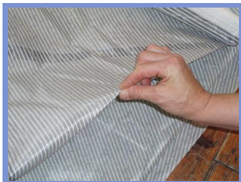
Figure K.1.1.2 soft sail which can be folded without damage
