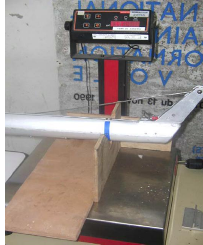
Mast weight / centre of gravity (left) and tip weight (right) measurement. The centre of gravity may be checked using a knife-edge to balance the mast.
