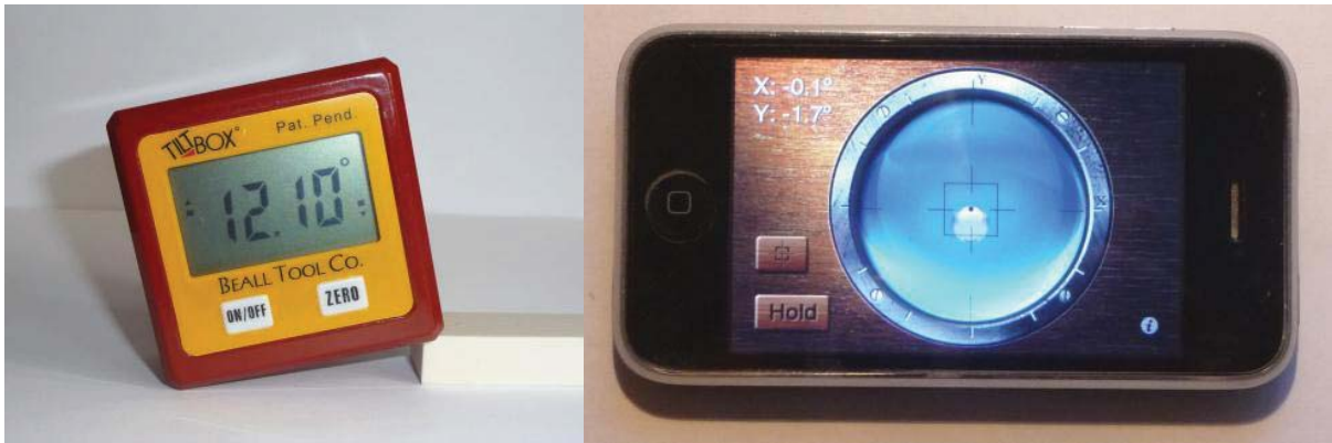
Figure F.6.5.2 A 0.05 deg. resolution inclinometer and the iPhone 0.1 deg. resolution level.
